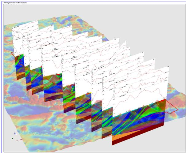
Figure 7. Forward gravity modelled, full crustal serial cross-sections over the Stavely Project area. Assigned density values have been constrained by MSCL density measurements where available. Background image is of high-pass filtered gravity data.
