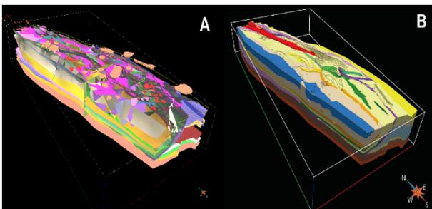
Figure 8. Stavely 3D geological model showing modelled A) surfaces and intrusives, and B) volumes. Spatial distribution and geometries have been informed by geophysical data, the interpretation of which has been constrained by petrophysical property values and their distributions.
