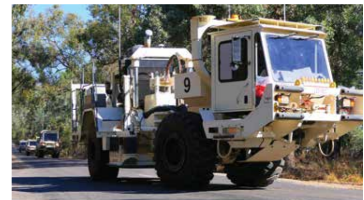
Figure 2. Seismic survey Vibroseis trucks in northeast Victoria. Photo: Geological Survey of Victoria.
