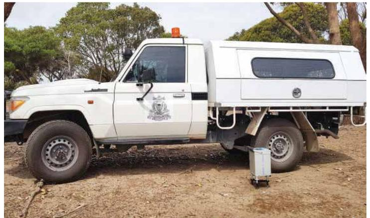
Figure 4. Geological Survey of Victoria vehicle with gravity meter. Photo: Geological Survey of Victoria.
